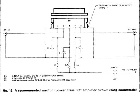
fig. 12. A recommended medium power class "C" amplifier circuit using commercial hybrids. Gain is approximately 30 dB and output is 7-12 watts with 100 milliwatts drive. See text for suppliers. Be sure to provide adequate heat sink with several radiating fins. Under normal operation the heat sink will have to dissipate up to 25 watts of power.
